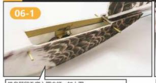
机身预留孔穿入圆木杆,如上图。 Insert the round wood rod into the reserved hole of the fuselage as shown above. 把机面放置到机身层中位置。用橡皮筋细定机面。(如上图底元
