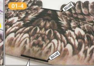
把粘合好的机魔反转到反面,在预留槽内嵌入碳片,用胶水粘牢固。 Reverse the bonded wing to the reverse side, insert the carbon sheets in the reserved groove, and glue it firmly with glue.
