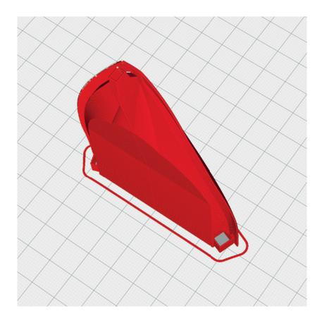
The following parts must be sliced with the PROFILE P3\_SURFACE (1-wall-print). Please note the additional settings for the individual parts!
